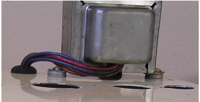
Guide all of the wires through the chassis. (Learn from our mistakes.) The extra wires will be secured and stowed inside the chassis. Their location outside the chassis is too susceptible to the heat from the tubes. Secure the output transformer to the chassis using the stock nuts & bolts that you kept !
