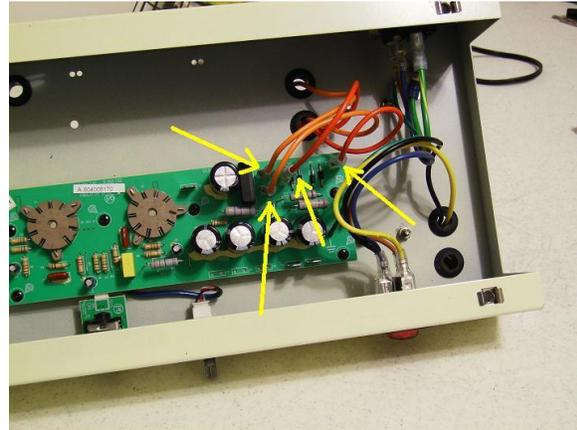
Remove the six (6) screws fastening the circuit board to the chassis. Keep them. You'll use them to attach the new PCB.
