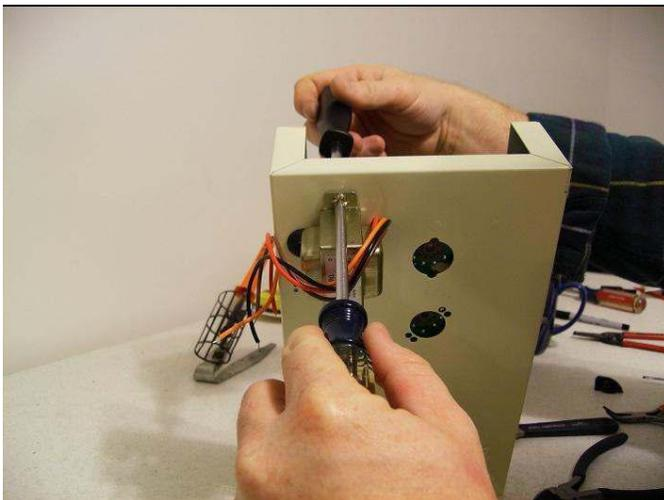
Keep the output jack board with its ground wire attached.
