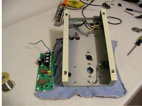
Salvage the ground wire from the stock circuit board for use later.
