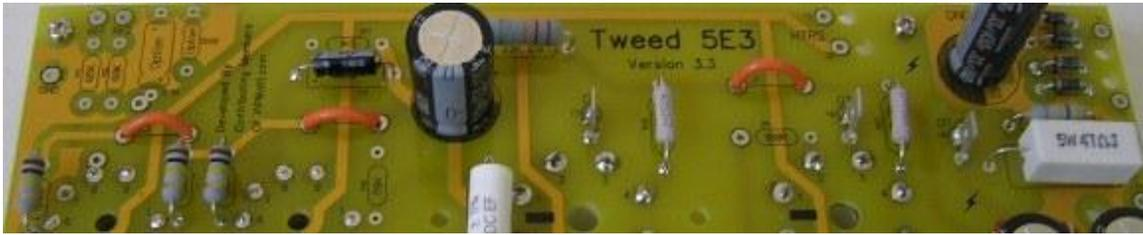
Finally, the last of the resistors ! Note that R7 & R8 are not installed on the PCB. They are part of the input jack complex.
