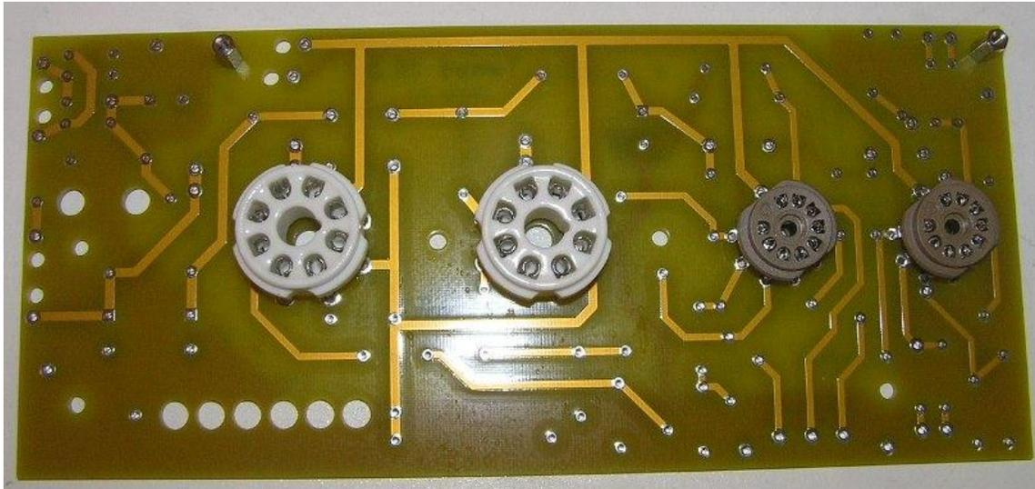
The tube sockets are installed as shown. The noval sockets only go in one way (on the back side). However, the octal sockets need to be properly oriented with the circuit board. Position the notch in these sockets so that they are pointing toward the two noval sockets.
