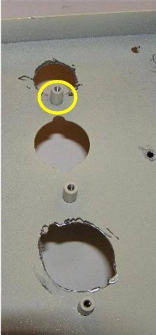
You want to drill the Noval (9-pin) holes so that the socket 'lip' rests against the chassis. The Octal (8-pin) socket holes need to allow the socket to slip all the way through.
