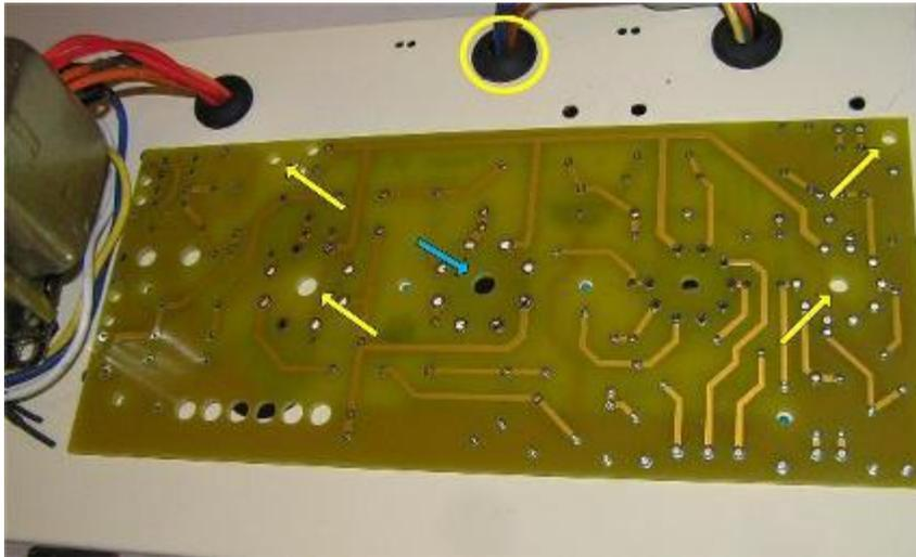
Mark the existing stand-offs so that you can use them to line up the PCB & then lightly tape it to the chassis.
