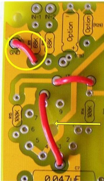
Don't forget the jumper to connect v1's pins 3 & 8 ! I did...
