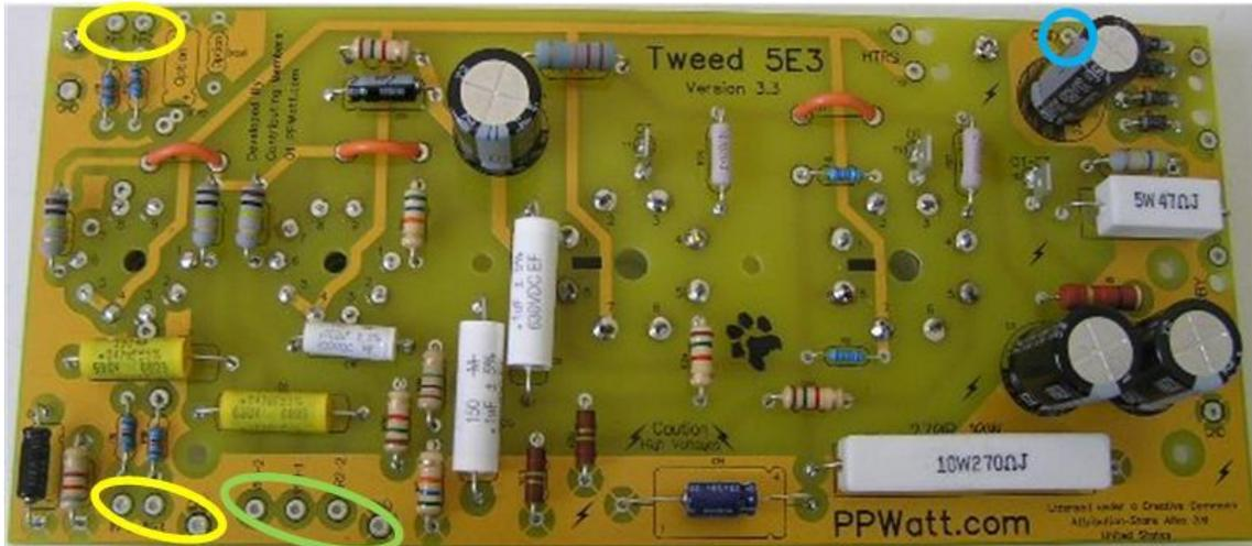
The input jack wires connect to the pads marked in yellow.
