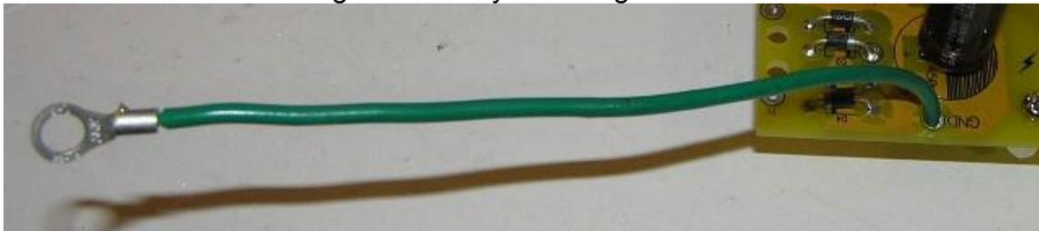
This will be connected to the existing ground post. You will note that the mains ground wire from the IEC connector also connects to this post. Some people say it is better practice to have a separate ground for that wire than the star ground for all the others.
