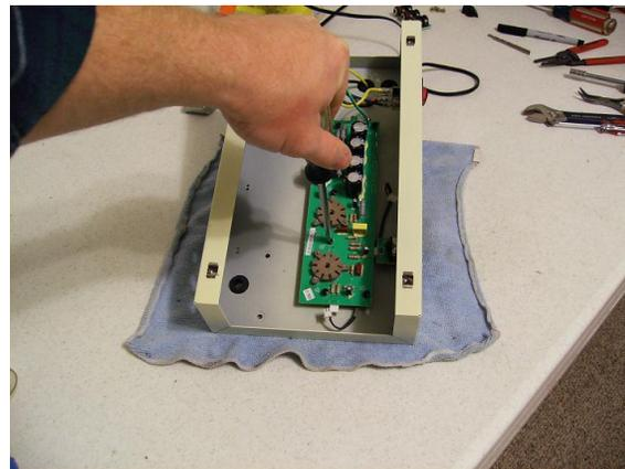
Remove the stock circuit board and pull all of the power transformer leads to the rim of the chassis.
