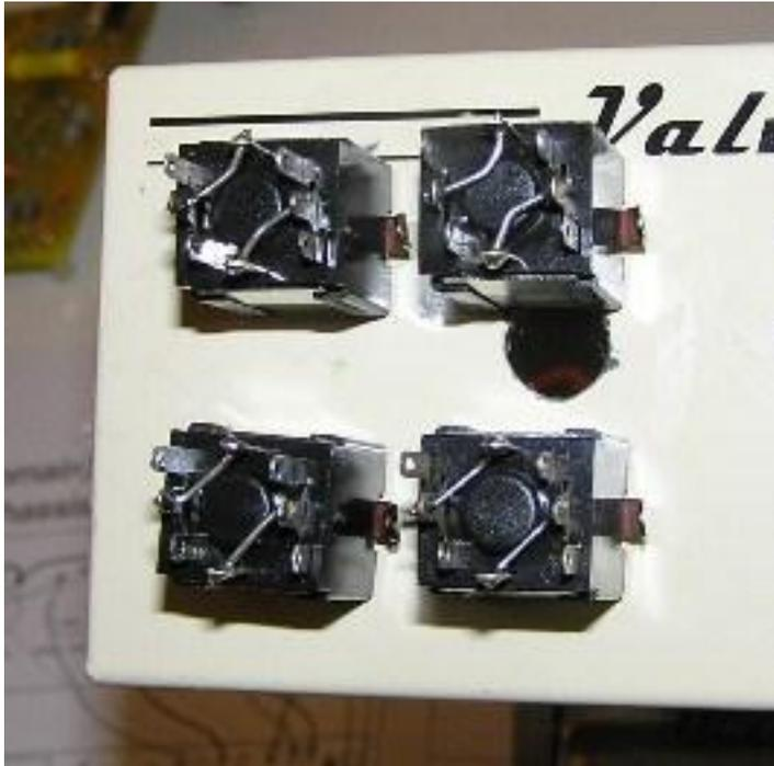
Look at the Chassis Layout diagram to see how you are going to wire together the input jacks. I find it easier to wire them together when they are connected to the outside of the chassis in their actual mounting holes.
