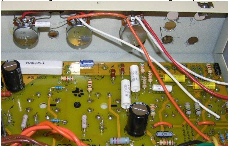
Mount the pots inside the chassis as shown: -
